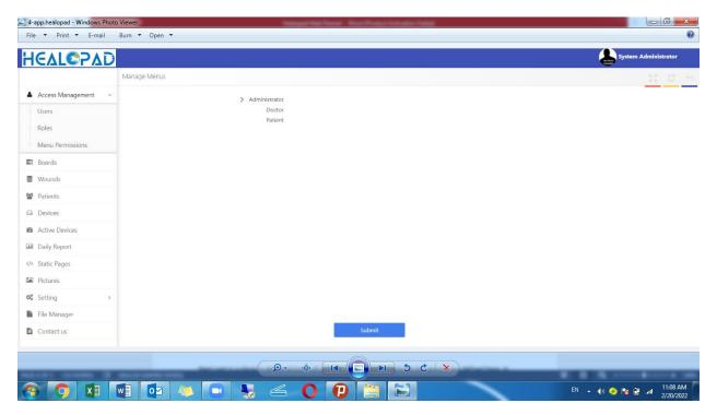
Next section is called Board. Here all the produced boards for the project, their serial number and their correspondent Mac Address should be defined, enabling the user's mobile to receive Mac Address data from server after serial number input and data transmit is ensured from the Pad to the mobile and then to the server.
